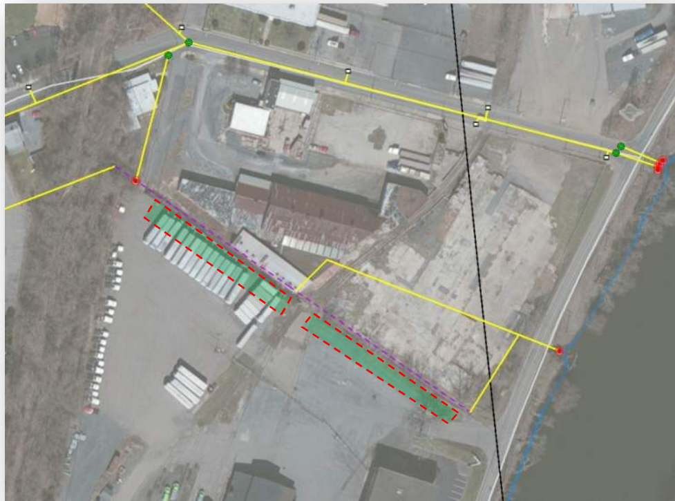
Mapping: Aerial view showing location of the vegetated filter strips above the open channel. Sections of impervious pavement shall be removed for the filter strip installation.
