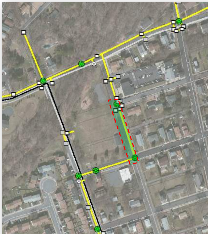
Mapping: Aerial view showing location of the bump out curb to provide a bioswale along the community park on Keystone Ave.
