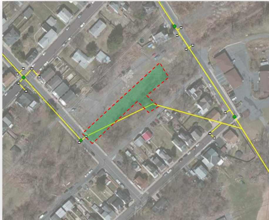
Mapping: Aerial view showing location of rain garden area within the Ridge Street property. A bioswale may be suited to accommodate the maintenance building footprint and site layout.
